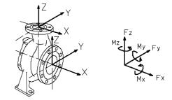
Forces and moments values are applied to the whole flanges and not flange-by-flange. For their sharing out on the pump flanges, refer to standard NFCR 13 931.
